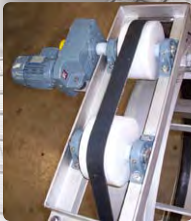
Simple and robust drum driving system.
