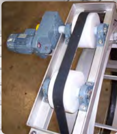
simple and robust drum driving system
